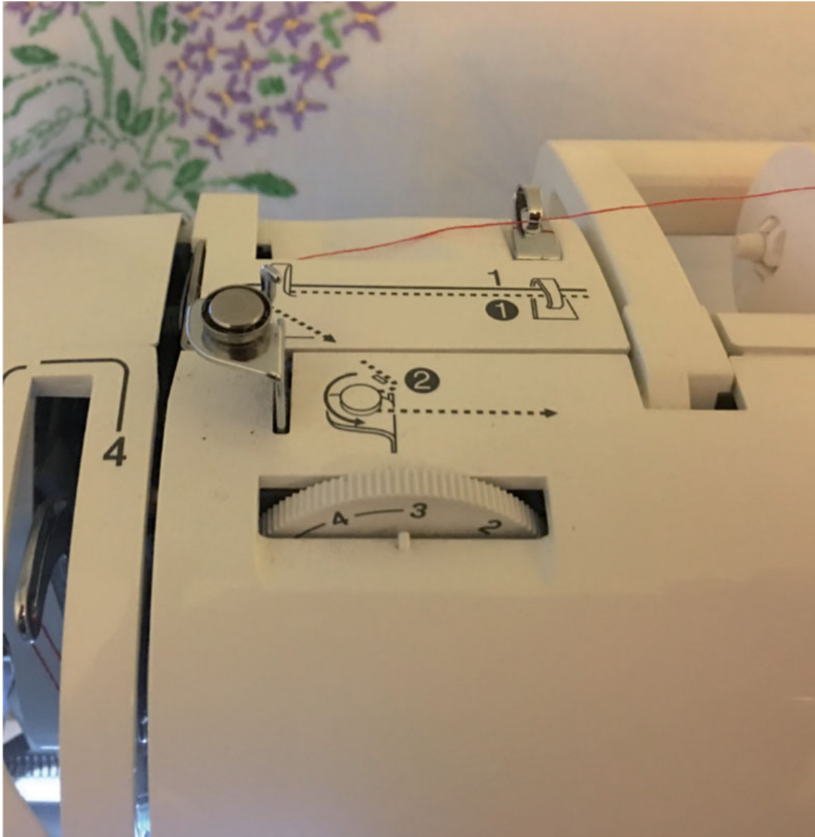
Fig. 15 Threading the machine using numbered markings.
