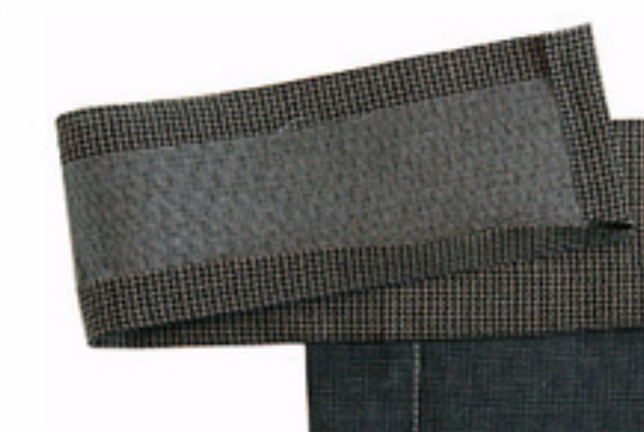
2. Press up the band and band/garment seam allowances, then fold the band over itself, right sides together.
