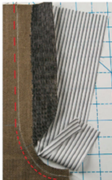
2. The crotch curve is stitched, and the center-front is basted.
