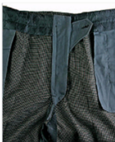
The band and garment seam is pressed open. A shield tab was added. The shield extends over the crotch seam, and the fork is stayed with the lining.
