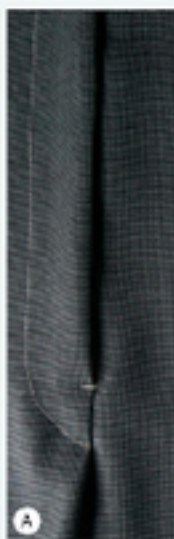
A and B: These crotch seam allowances are pressed toward the overlap and caught in the overlap topstitching.
