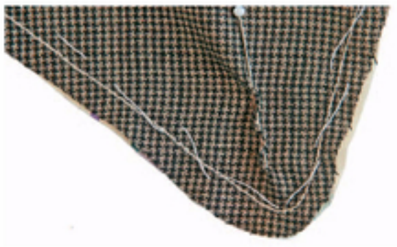
A pin inserted at a corner fold gathers a little ease
