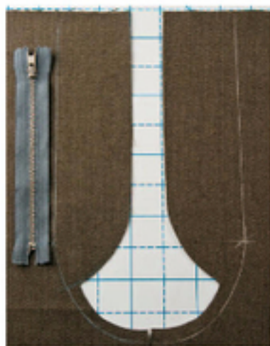
Here's a fly with cut-on extensions, all marked up and ready to go.
