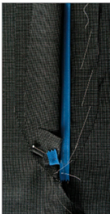
8. Here's the underlap facing basted in position, with the shield and left zipper tape folded out of the way.
