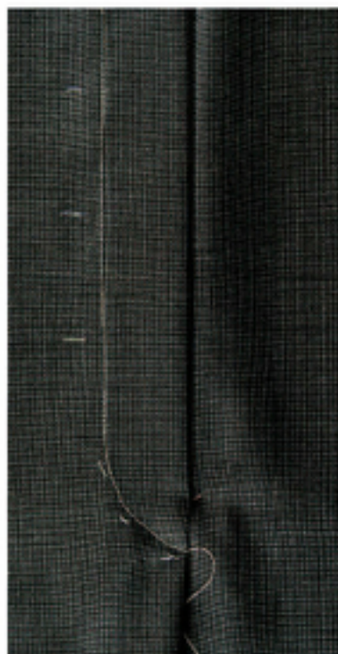
9. The basting stitches help guide the topstitching.
