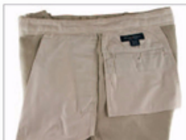
The soft-lined band catches the pocket bags. The front bags are finished with the side seams.
