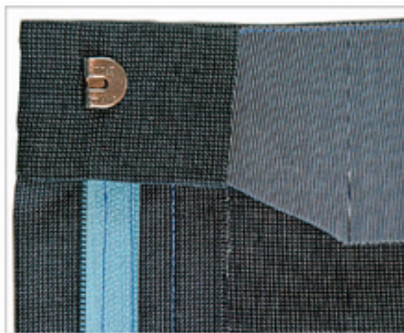
10a. The petersham can fold within the extension if the seam clip is moved away from the front.
