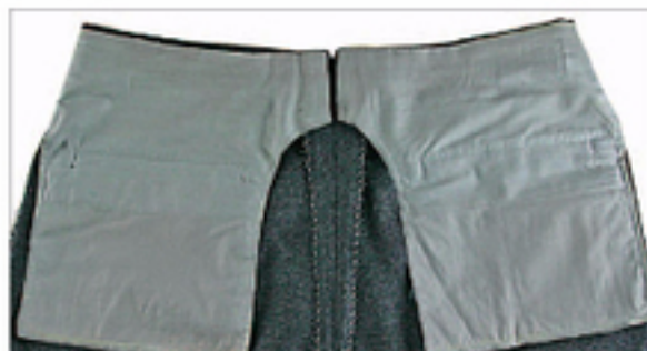
The pocket bags finish the band. The center-back seam allowances are overcast-stitched by hand. The split band at center back allows for ease of movement.
