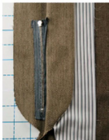
4. The zipper tape is stitched to the overlap with two rows of stitching.
