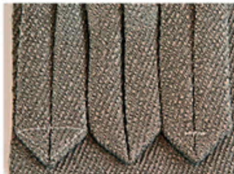
Here are three topstitching options: triangular stitching, hidden stitching, and simple tacking.
