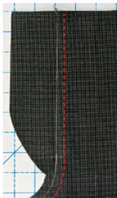
2. The crotch curve is stitched, and the center-front opening is basted.
