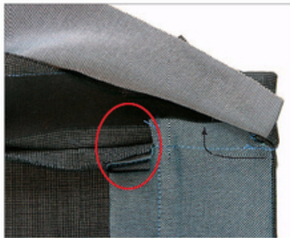
4. The band and lining are turned to the inside. The arrow indicates where to press allowances above the fly. The circle shows the clipping that allows the opening of the seam beyond the fly.
