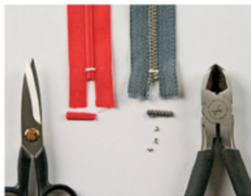
Unwanted teeth, either plastic or metal, can be easily cut away. Metal teeth can also be removed individually with nipping pliers.
