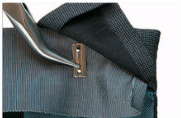
6a. Needle-nose pliers help you bend down the eye's prongs.
