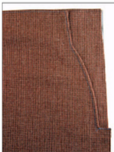
This slant-top pocket is not joined to the facing at the waist.
