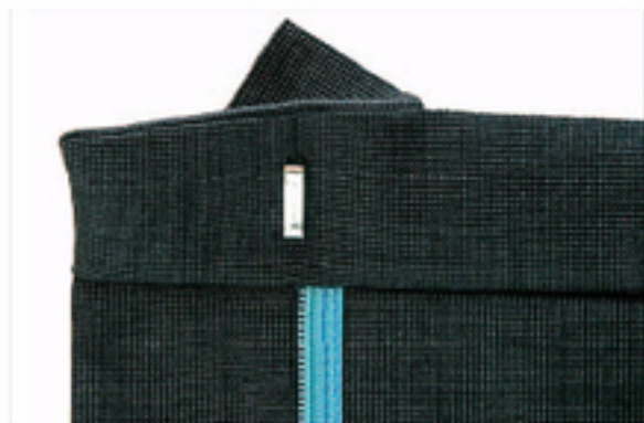
6. Position the clamp-on eye above the underlap zipper teeth.
