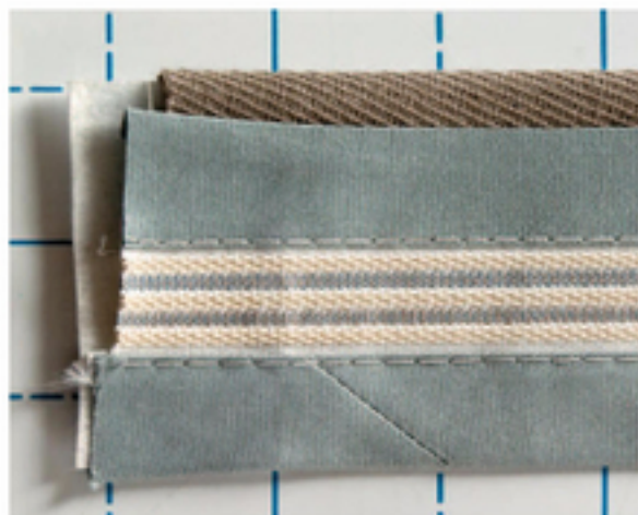
The band fabric is folded over the waistband layers.
