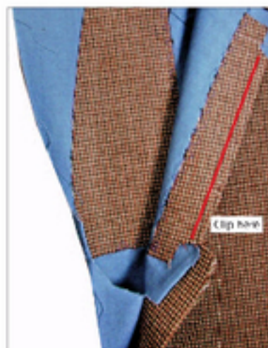
Clip the pocketing fabric just below the pocket mouth. Topstitch the mouth edge.
