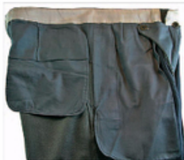
The curtain, which covers the band/garment seam, is inserted only in back. In front, it's replaced by pocket bags.
