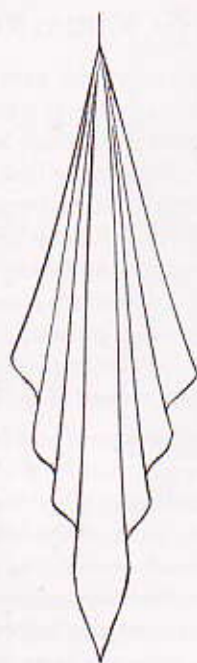
Fig. 5-5. Square godet creates a handkerchief edge. The floating corner and sides of the godet can be adjusted for length.
