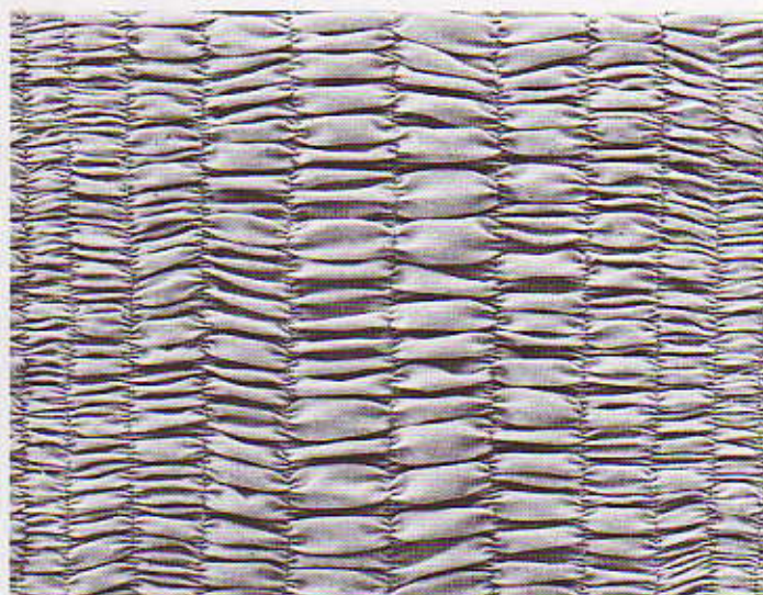
II-2—Machine-stitched shirring gathered on bobbin threads.
