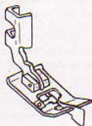
Fig. 3-17. Medium-to-wide satin-stitched edgings lie flat when sewn with an overedge foot.
