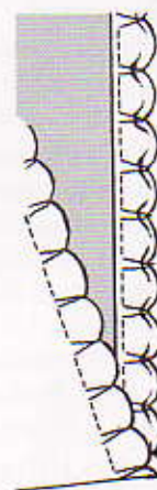
Fig. 3-11. Machine-stitched shell hem shaped by an overedge stitch with needle-thread tension increased.
