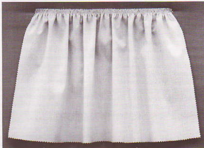
1-2—Muslin gathered moderately full on machine-sewn stitching loses 50% of its original length.
