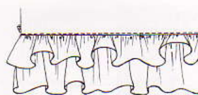
Fig. 3-33. Two ruffles, the upper ruffle shorter than the ruffle underneath, applied as one to the fabric's edge.
