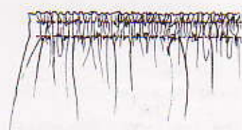
Fig. 1-3. Fabric gathered on two rows of hand or machine stitching.
