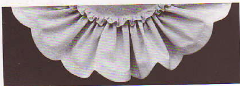
III-6—Layered ruffles. The narrow ruffle on top, gathered from a strip cut two times the target length, was finished with a zigzagged flat hem. The wide ruffle underneath, gathered from a strip cut three times the target length, was finished with a faced, scalloped edge.
